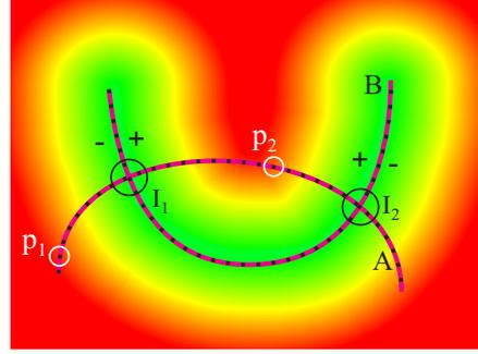
Figure 3: Two point clouds  $A$  and  $B$  and their intersection spheres  $I_1$  and  $I_2$ . Our root finding procedure, when initialized with  $p_1, p_2 \in A$ , will find an approximate intersection point inside the *intersection sphere*  $I_1$ .
