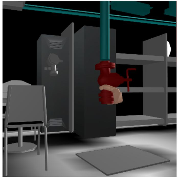
Figure 12. NEW PIPES CAN BE DESIGNED FROM BUILDING BLOCKS. HERE THE USER ATTACHES A VALVE TO THE END OF A NEW PIPE. WHEN THE VALVE TOUCHES THE PIPE AND IT HAS NEARLY THE “CORRECT” POSITION, THE SYSTEMS SNAPS IT TO THE PIPE. DURING POSITIONING, COLLISIONS BETWEEN VALVE AND PIPE ARE HIGHLIGHTED BY RENDERING THE PIPE IN WIRE-FRAME. (DATA COURTESY .)
