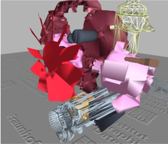
Figure 11. DURING AN INTERACTIVE FITTING SIMULATION IN A VIRTUAL ENVIRONMENT, THE SYTEM HIGHLIGHTS ALL OBJECTS COLLIDING WITH THE ALTERNATOR (DATA COURTESY AIT CONSORTIUM).
