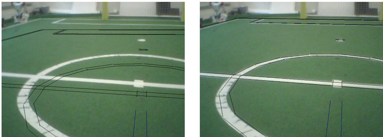
Figure 4.4: Camera calibration using *calibrationHelper*: Projected lines before (left) and after (right) the calibration procedure
