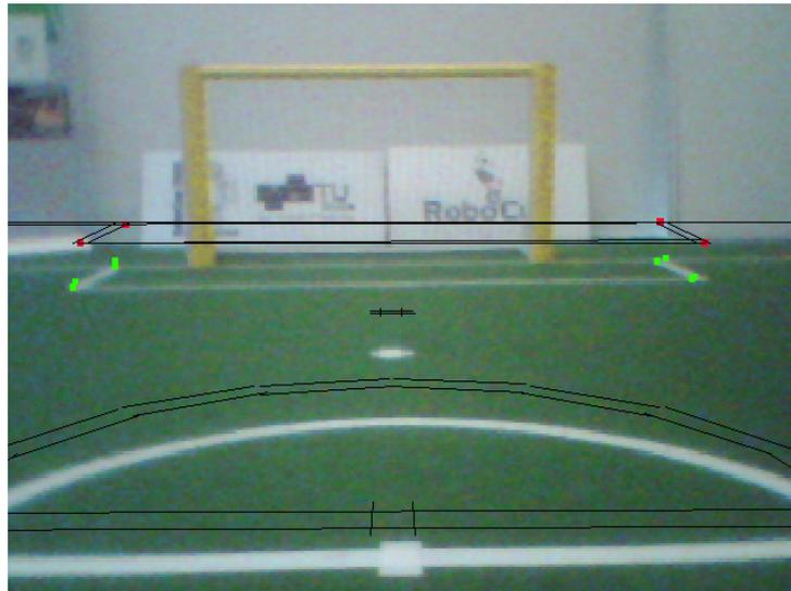
Figure 4.5: Camera calibration using CameraCalibrator: Projected lines during calibration procedure
