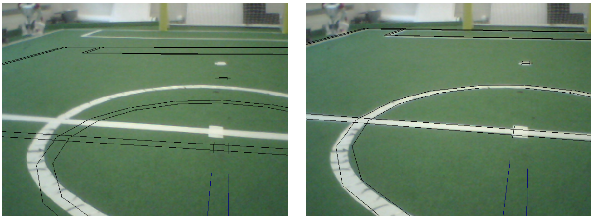
Figure 4.4: Camera calibration using calibrationHelper : Projected lines before (left) and after (right) calibration procedure
