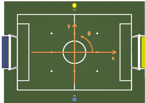
Figure 4.2: Visualization of the global coordinate system
