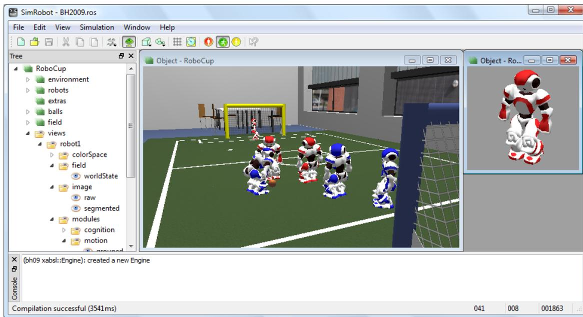
Figure 7.1: SimRobot with the tree view on the left and two scene views on the right. The console window is shown at the bottom.
