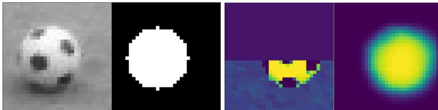
Fig. 3: Training ball segmentation. The left image shows a training example, the right image shows an exemplary inference result.
