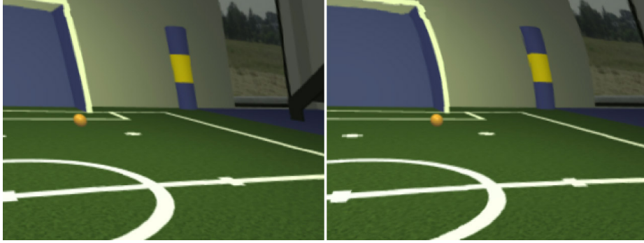
Fig. 2. Examples of image distortion for a rolling shutter simulation based on per-pixel velocity. The left image has been generated using a constant velocity, whereas interpolated velocities have been applied to the right image.
