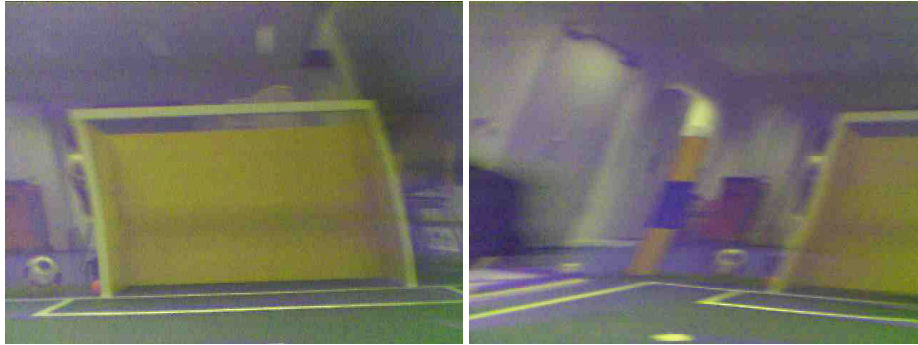
Fig. 1. Examples of image distortion caused by the rotation of a CMOS image sensor with a rolling shutter.
