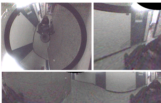
Figure 4: Omni directional camera view (top left); Unwarped perspective view (top right) and panoramic view (bottom). Corresponding to the situation presented in Fig. 3 right.
